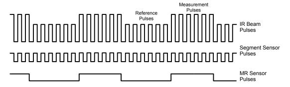
Figure 13-12: Segment Sensor and M/R Sensor Output
